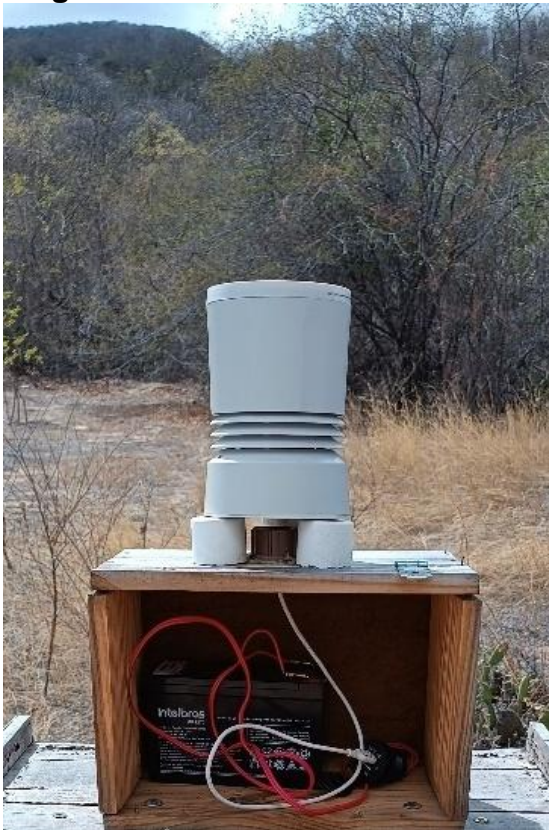
Figure 03 – Installation of the THP3
